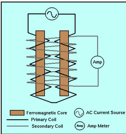
Figure 30 - A diagram showing one type of fluxgate magnetometer. A primary coil is wound around the iron bars and an alternating current is run through this wire. A secondary coil is wrapped around the iron bars to measure any changing magnetic fields due to magnetic saturation of the iron bars. An external magnetic field aligned parallel with the bars will influence the signal measured by the secondary coils. Some fluxgate magnetometers use rings of iron instead of bars.
