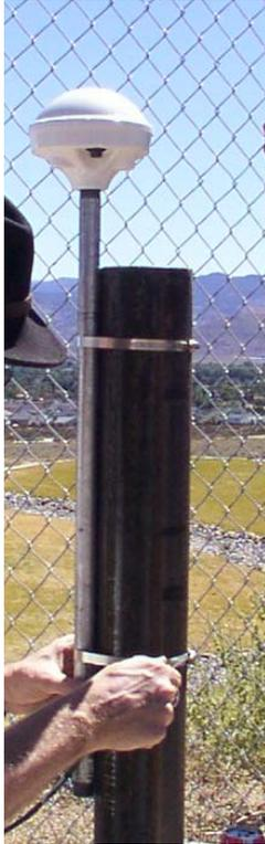
**Figure 32** - White GPS antenna being attached to a pipe at the Carson City, Nevada site. Usually it is better to have the GPS away from fences, but this one had a big enough field-of-view in the other direction to get data from the GPS satellites.
