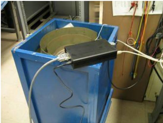
**Figure 33** - Magnetometer electronics box (black box) sitting on a blue magnetic shield test can. Three wires come into this box: one is attached to the magnetometer sensor, one to the GPS, and the third is attached to the computer.
