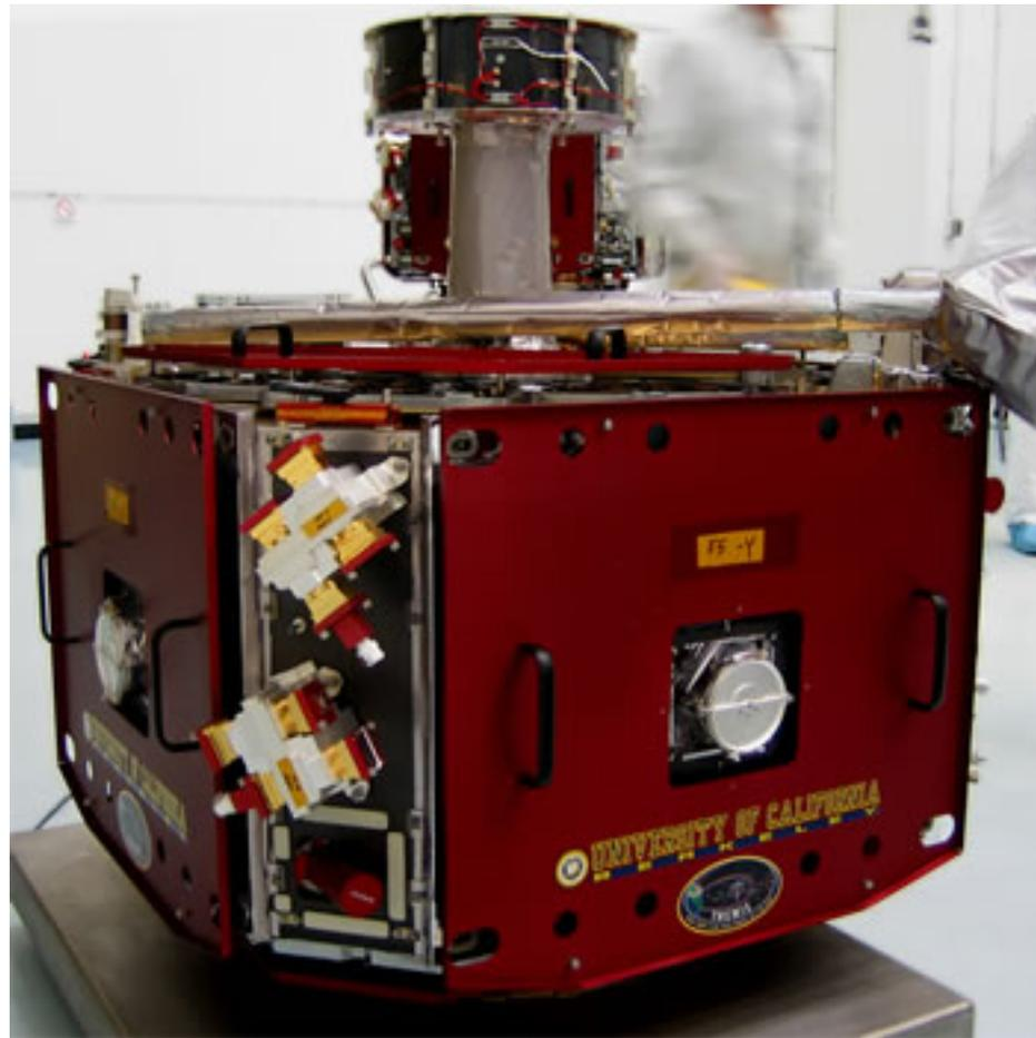
One of the five THEMIS spacecraft prior to launch. Its two solid-state telescope units, each with two opposite-facing SSTs incorporating four silicon detectors each, are mounted on the near edge.
