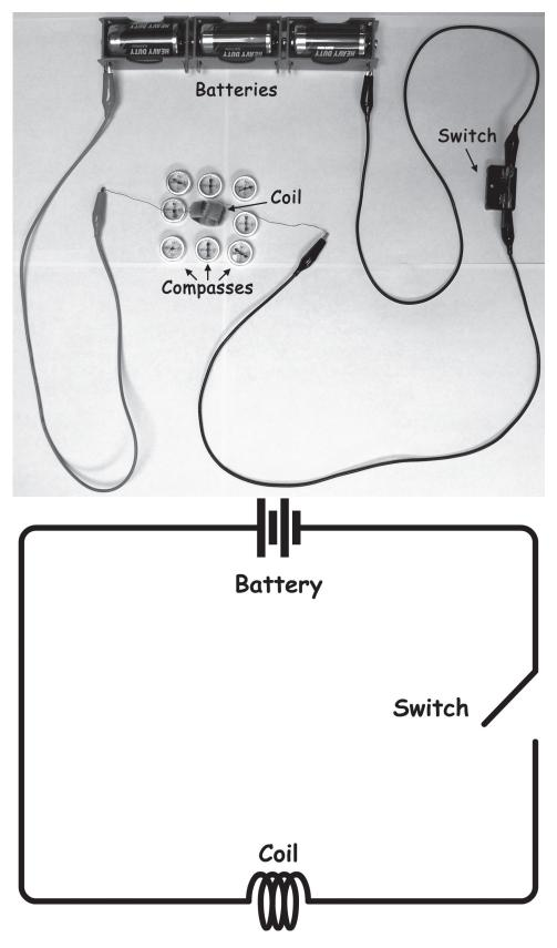
Figure 2.3: An electrical circuit with a coil of wire included. Compasses placed around the coil will detect any magnetic fields produced by the electrical current.
