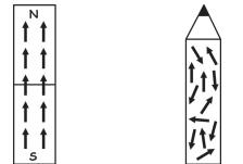
Figure B.1: Cartoon of atom's magnetic dipole fields in a bar magnet and in a pencil.
