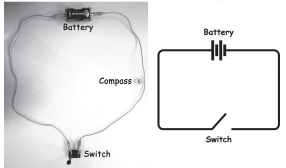
Figure 2.1: A simple electrical circuit
