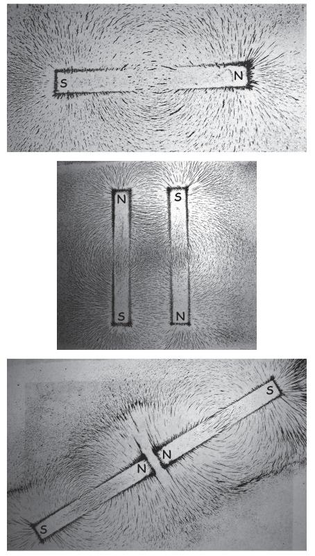
Figure 1.3: Iron filings on thin sheets of paper over bar magnets.
