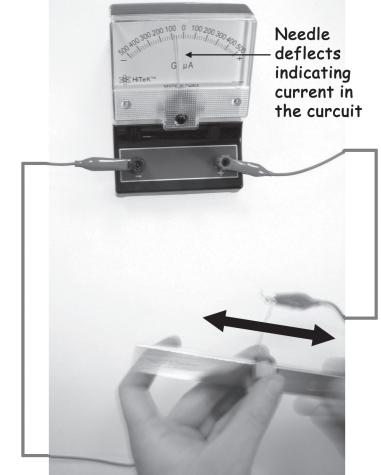
Figure 2.9 : Moving a magnet through the coil of wire produces a current. Blurry elements in the figure are an effect of this mothion being photographed.
