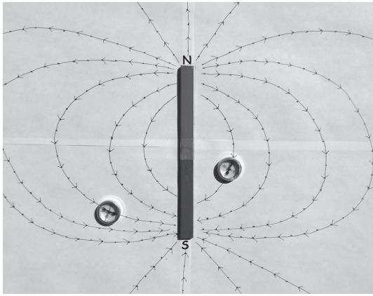
Figure 1.2: Magnetic Field line tracing of a bar magnet with a dipole magnetic field using compasses.
