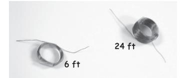
Figure 2.2 : Coils of wire, taped together. On the left is a 6-foot length of wire, on the right is a 24-foot length of wire.
