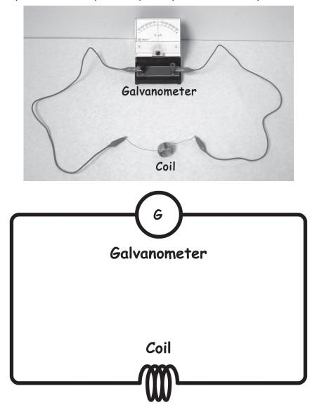
Figure 2.8 : Coil of wire in an electrical circuit with a galvanometer
