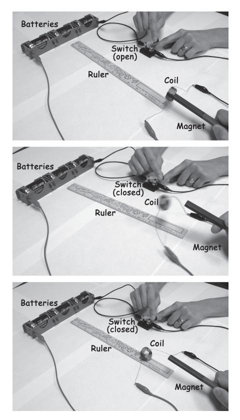
Figure 2.7: Set-up for the Jumping Coils Experiment
