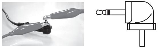
Figure 2.4 : Configurations for using an AC to DC adapter as a power source in the electrical circuit. Configurations will vary depending on the type of adapter plug. For the adapter shown, positive and negative terminals are on the outside of the plug separated by a plastic insulator.
