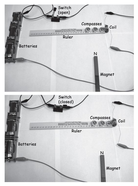
Figure 2.6: Set-up for the experiment with compasses aligned along the axis of a coil of wire.
