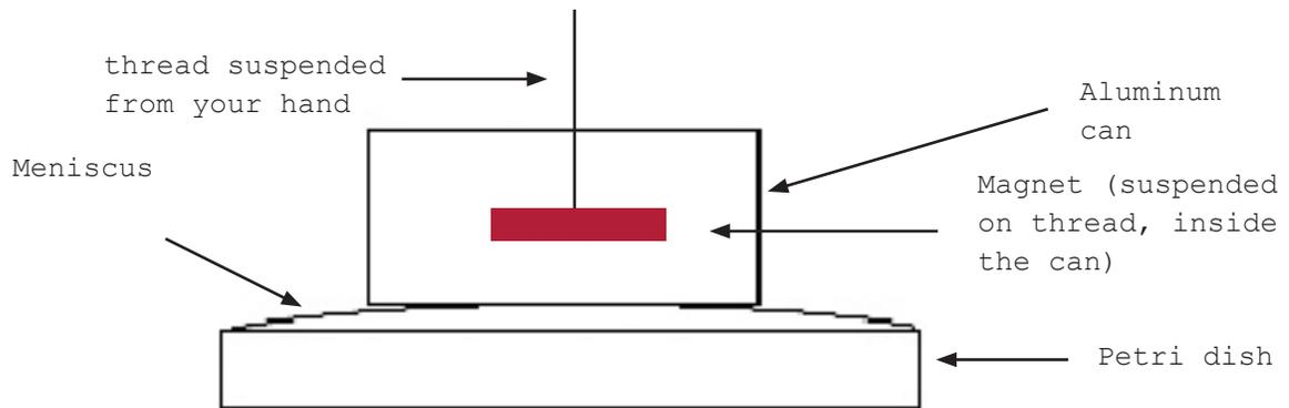
3. The length of thread should be tied to the center of the magnet so that it hangs straight. When you dangle the magnet into the can, the magnet should also be at least one inch shorter than the diameter of the can so that it does not bang into the sides of the can while students attempt to spin it.
