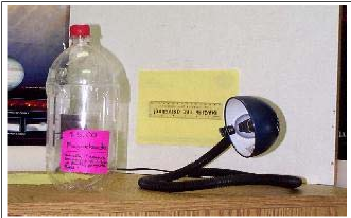
Figure 30 - A soda bottle magnetometer and its setup. The lamp illuminates a mirror on the suspended magnet, and creates a spot on the wall, whose displacement is measured by the ruler.
