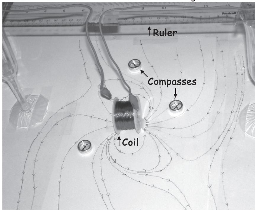
Figure 2.5: Here the entire spool of wire is used as a coil in an electrical circuit. The glasses and ruler are used to hold the wires off the table so that a tracing of the magnetic field around the coil can be drawn on the paper beneath it.
