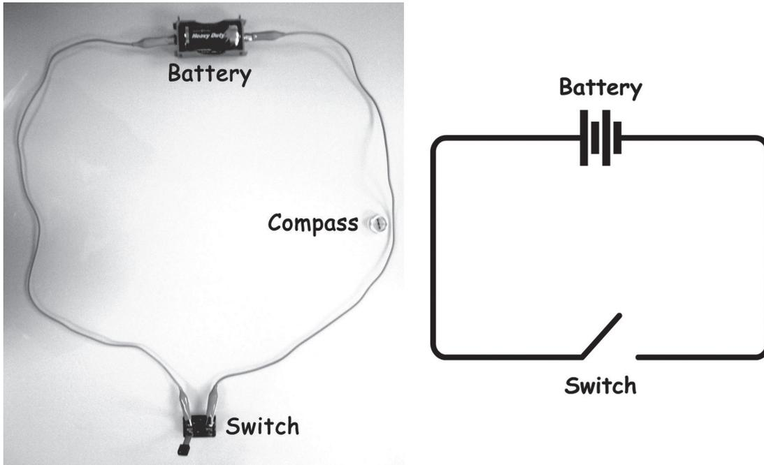
Figure 2.1: A simple electrical circuit
