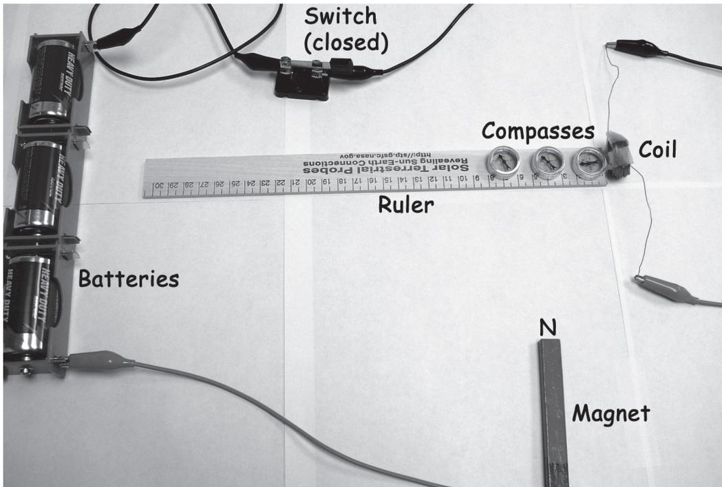
Figure 2.6: Set-up for the experiment with compasses aligned along the axis of a coil of wire.
