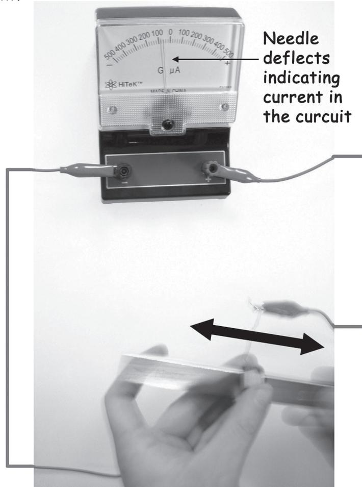
Figure 2.9 : Moving a magnet through the coil of wire produces a current. Blurry elements in the figure are an effect of this motion being photographed.
