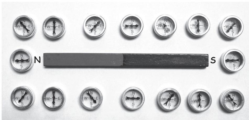
Figure 1.1: Bar Magnet with magnetic compasses placed around it. Note how the heads of the compass needles point toward the magnetic south pole and away from the magnetic north pole of the Bar Magnet.
