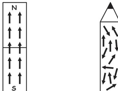
Figure B.1: Cartoon of atom's magnetic dipole fields in a bar magnet and in a pencil.
