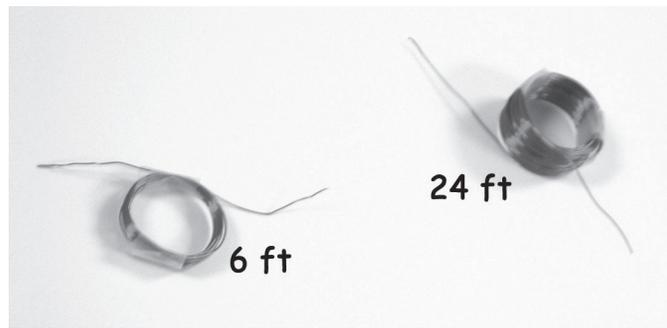
Figure 2.2 : Coils of wire, taped together. On the left is a 6-foot length of wire, on the right is a 24-foot length of wire.
