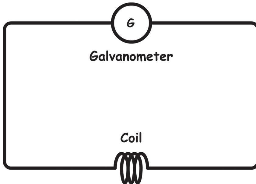
Figure 2.8 : Coil of wire in an electrical circuit with a galvanometer
