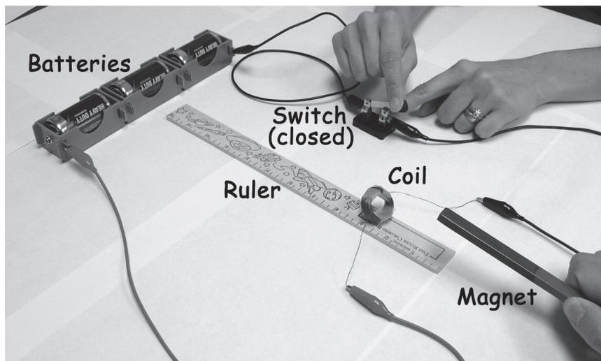
Figure 2.7: Set-up for the Jumping Coils Experiment
