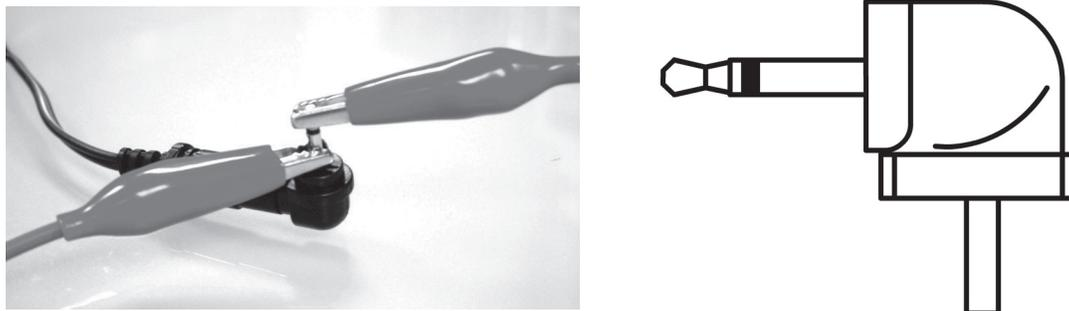
Figure 2.4 : Configurations for using an AC to DC adapter as a power source in the electrical circuit. Configurations will vary depending on the type of adapter plug. For the adapter shown, positive and negative terminals are on the outside of the plug separated by a plastic insulator.
