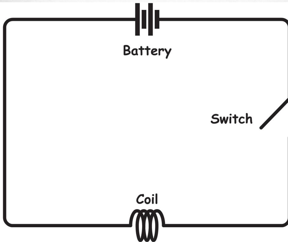
Figure 2.3: An electrical circuit with a coil of wire included. Compasses placed around the coil will detect any magnetic fields produced by the electrical current.
