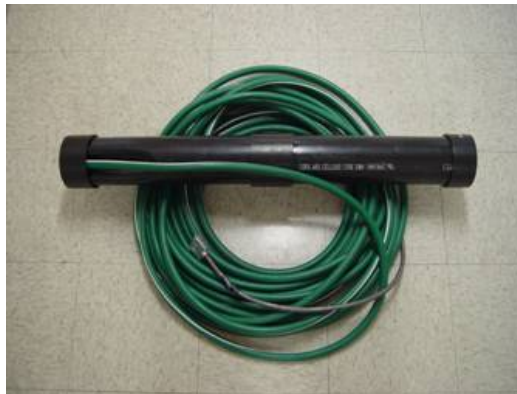
Figure 31 - Magnetometer sensor located in the black tube, with the sensor cable located inside a garden hose for protection against chewing little creatures.
