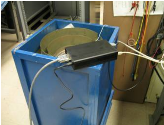
Figure 33 - Magnetometer electronics box (black box) sitting on a blue magnetic shield test can. Three wires come into this box: one is attached to the magnetometer sensor, one to the GPS, and the third is attached to the computer.
