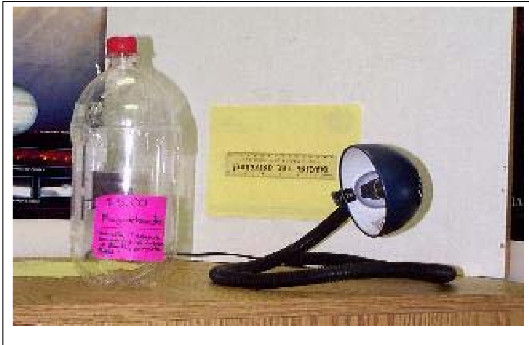
Figure 29 - A soda bottle magnetometer and its setup. The lamp illuminates a mirror on the suspended magnet, and creates a spot on the wall, whose displacement is measured by the ruler. For more accurate measurements, a laser pointer can be used, attached securely to a stand (test tube holder) so that the pointer-soda bottle system does not move during the course of the measurement program. This can be built with simple woodworking skills.
