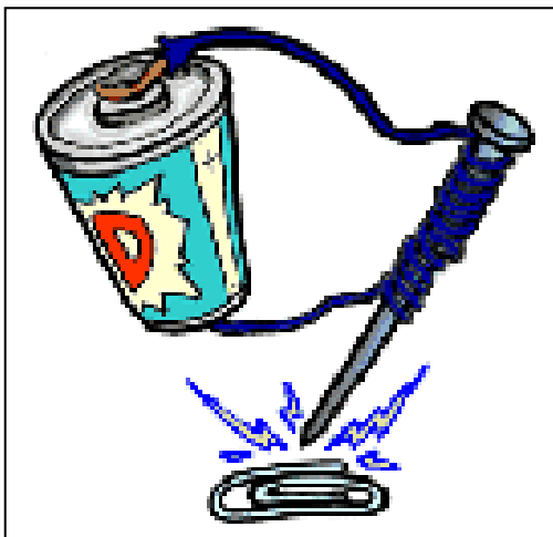
Figure 5 - Current flowing in a wire creates an electromagnet as shown in this cartoon sketch. The nail amplifies the magnetism enough for it to pick up a few metallic paperclips.
