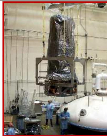
**SIRTF CTA is lifted into the 'Brutus' test chamber**
